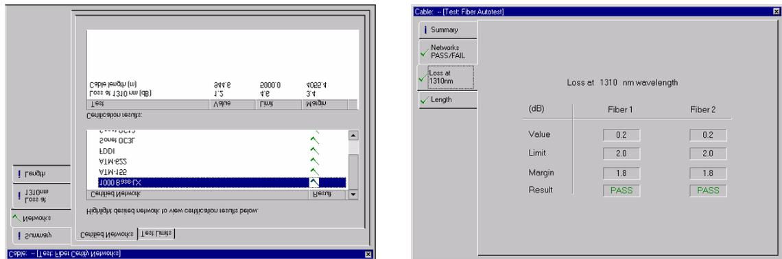
Figure 3: A sample test report displaying application-specific pass/fail results for each fiber optic network (left) in addition to the generic TIA and ISO pass/fail results for cable loss (right).
